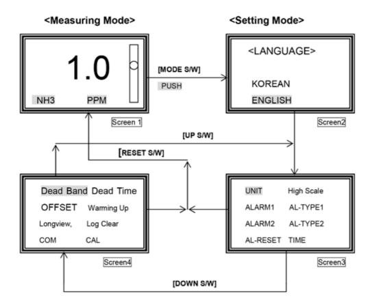
Please press MODE key longer than 3 seconds in measuring mode to enter into setting mode. (Screen1)
