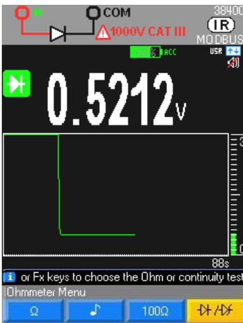
Reading of the threshold voltage; if the circuit is open or the threshold of the diode >4V, the indication is OL.
