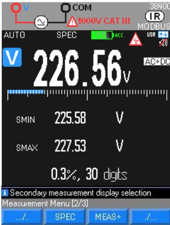
Using the internal technical specifications of the multimeter, the **SPEC** mode directly displays the tolerance on the measurement in progress, with no need to look for it and calculate it.
