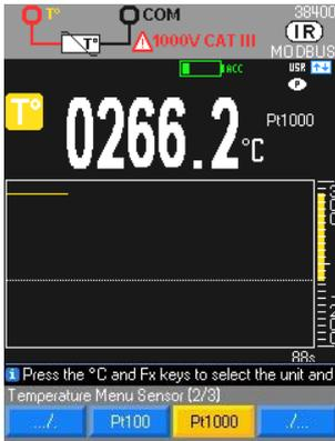
Measurement of the temperature with a sensor: Pt100/Pt1000.
