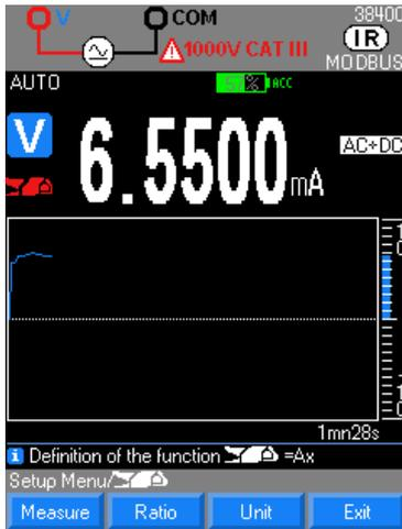
1. Activate the clamp function and, depending on the type of clamp connected, double-press "Clamp" or use the setup/clamp menu specify the coupling.
