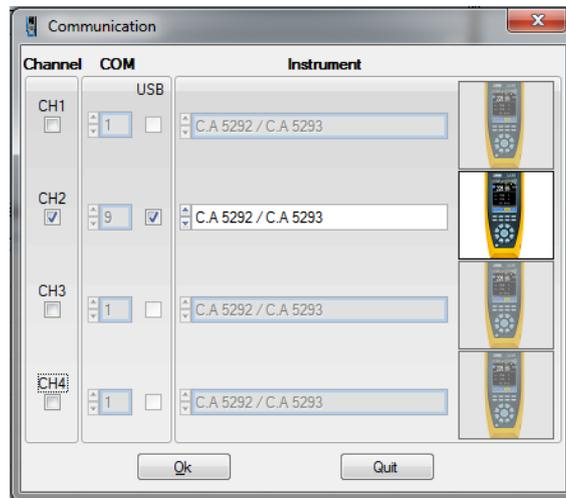
With some Bluetooth adapters, a reboot of the PC is recommended to validate the connection. The connection parameters are specific to each multimeter. They must be assigned manually, the first time only.
