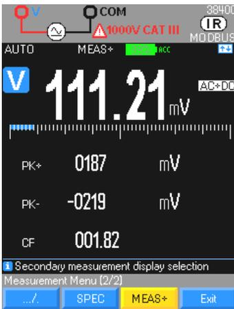
The rapid peak measurements are available in the **MEAS**, **MEAS+**, **PK+** and **PK-** secondary measurements for the following measurement functions: V and A (AC, AC+DC); integration time less than **250µs**.
