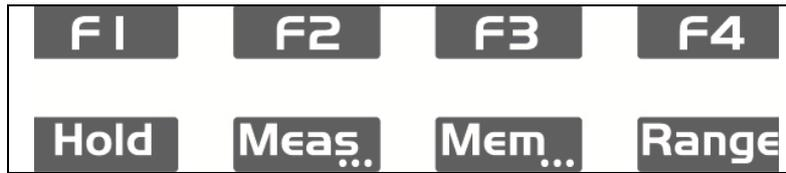
The keys are taken into account and applied when pressed. If the key press is validated, the instrument beeps. The active keys on a long press are identified by "...": **Meas...**, **Mem...**, **Setup...**
