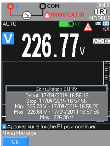
1. Press on the V function, then select the coupling according to your measurements: AC, DC, AC+DC, LowZ (AC is default).
