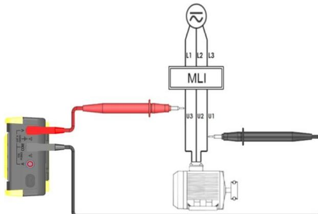
**Connecting the multimeter to filter a current >300Hz**
