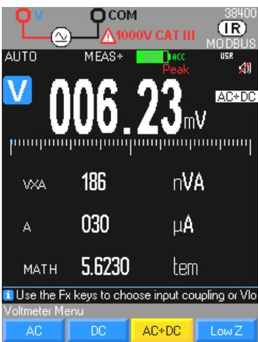
The power calculation **VxA** (VA) requires a third connection on the A input (connected to the same circuit), in order to measure simultaneously:
