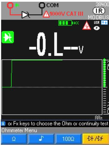
Zener diode or LED: selecting this diode applies the same function as for the diode above but with a maximum voltage of 26V and a maximum current of 10mA.
