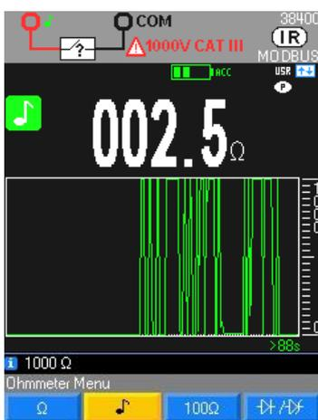
Measurement of a resistance up to 1000Ω , with continuous 4kHz audible indication.
