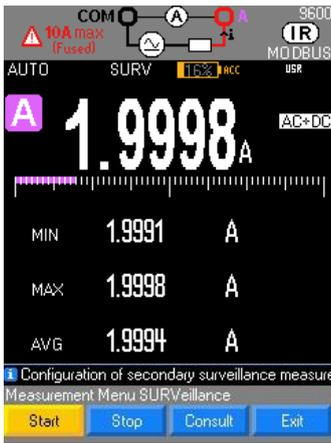
1. Press function A, then select the coupling according to your measurements: AC, DC, AC+DC (AC+DC is default)
