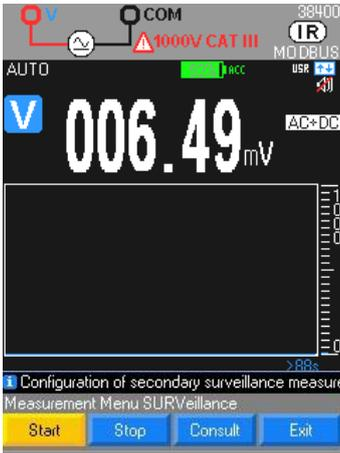
Integration time at least **200ms**, programmable according to your configuration: **Start** → **Stop**, then look-up of the quantities on the screen, in a specific window.
