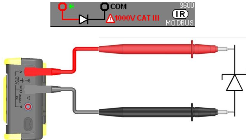
This function performs a diode forward voltage check to verify:
