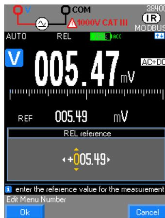
This mode indicates that the value displayed is relative to a reference value. It is available for the following measurement functions: V, Hz, Ohm, clamp, capacitance, temperature, and current.
