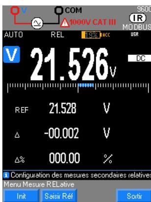
In the "DC" mode, you measure a direct voltage or the DC component of an AC voltage.
