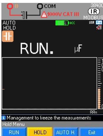
Measurement of the capacitance of a capacitor with a resolution of 1000pts "Run" appears when the measurement is in progress.
