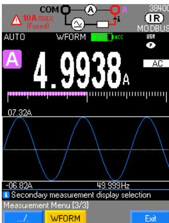
During an AC current measurement, the waveform of a signal at a frequency between 10 Hz and 600 Hz can be viewed using the **WFORM** function
