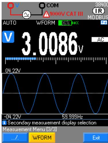
During an AC voltage measurement, the waveform of a signal at a frequency between 10 Hz and 600 Hz can be viewed using the **WFORM** function.
