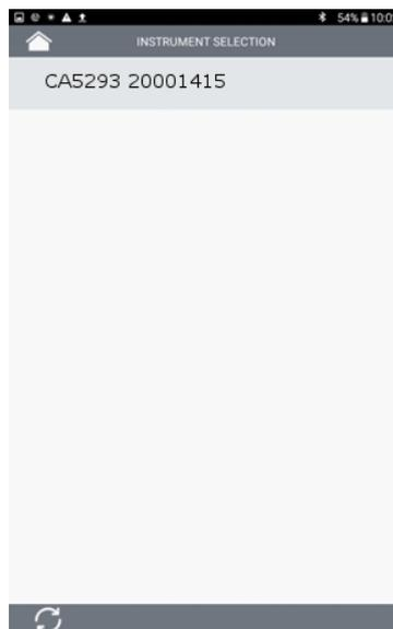
Activate the Bluetooth function and the MODBUS protocol on the multimeter. The connection is initiated by pressing the name of the instrument when it is displayed.
