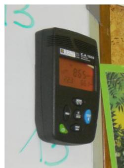
**Large number of mounting options:** magnetic, with padlockable wall support, with desktop stand or hung on wall hook.
