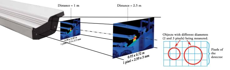
**Note:** The size of the measured object must be at least 3 x 3 pixels to guarantee precise temperature determination. This ensures that at least one pixel of the detector is completely covered (illustrated below).
