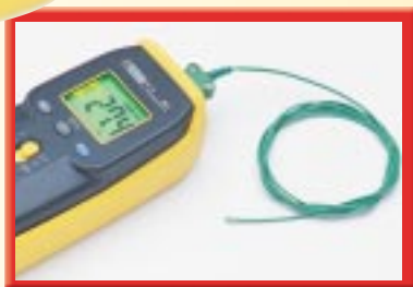
Delivered with 1 K-type thermocouple flexible sensor
