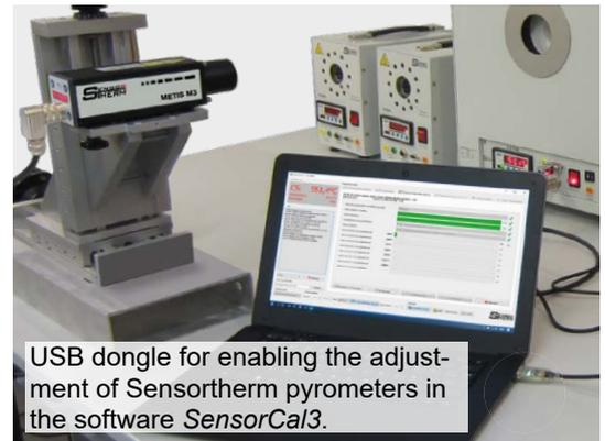
USB dongle for enabling the adjustment of Sensortherm pyrometers in the software *SensorCal3*.
