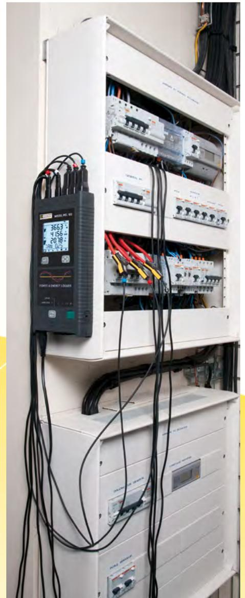
The monitoring by the PEL100 provides the recordings which will be compared with the reference.
