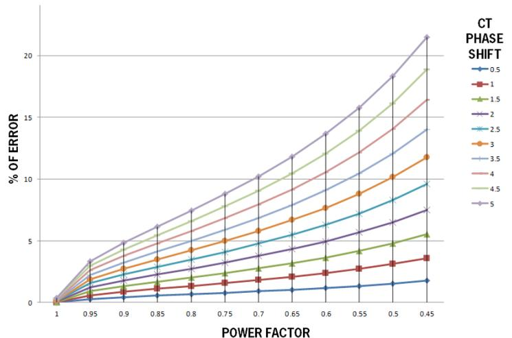
For example, with an uncorrected 3° phase angle error and reported power factor of 0.5, there is a corresponding kW error of >10%.
