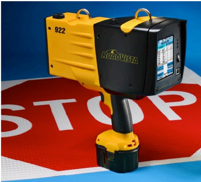
Reliable and field-proven, the 922 platform delivers a simple, economical solution for improving and maintaining roadway safety by providing a zero error means of assessing reflectivity data and inventory management control.
