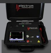
The MINI has one High Voltage lead that can be energized and two ground leads. The leads are moved between tests.
