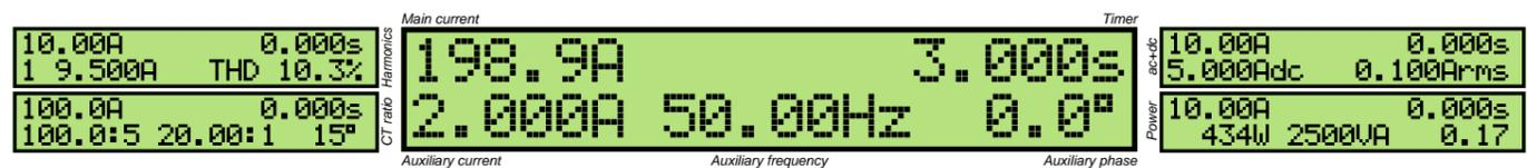
The 200ADM-P has a flexible auxiliary ac output that can be used at up to 260V for voltage relays or up to 10A for current relays. The phase and frequency of this output are fully adjustable. This combination of voltage and current allows testing of relays that require two voltages, one voltage and one current or two currents.
