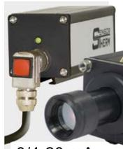
0/4–20 mA, RS232 or 485, switch input (clearing peak picker manually)
