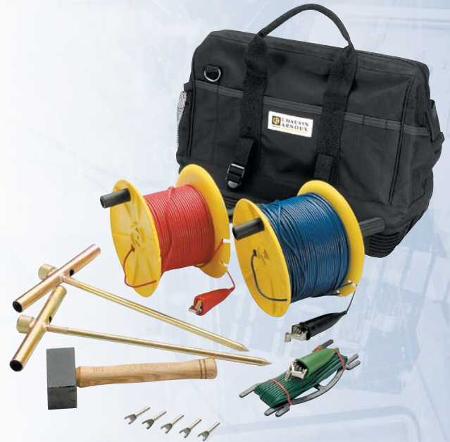
Earth kit: for measuring existing earth resistances using the 3-pole method (Standard carrying bag)
