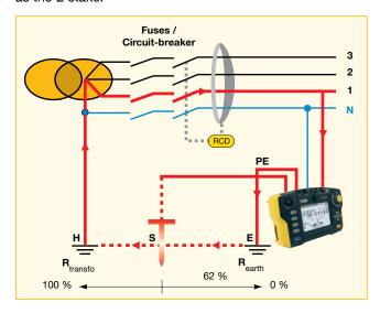
The measurement principle is the same as for the normal 62 % method.
