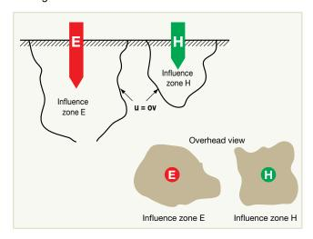
As diffusion of an electric current depends on the soil resistivity, it is difficult to be sure that the zones of influence have been avoided. The best way of confirming the measurement is therefore to repeat it after moving the stake S so that you can make sure it is similar to the earlier measurement.
