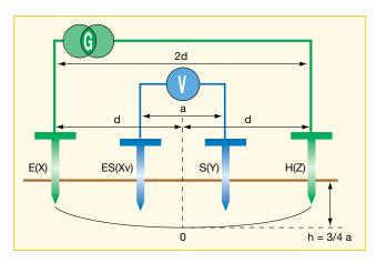
Although the Schlumberger method saves time, the Wenner method is better known and more widely used. The mathematical formula necessary is also much simpler. Nevertheless, many Chauvin Arnoux measurement instruments include both formulae for instant calculation of the resistivity values with either method.
