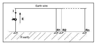
If the voltage E is applied to any point of the Rx earthing system, a current I flows in the loop in accordance with the following equation:
