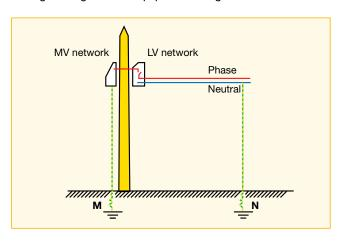
If lightning strikes the MV/LV transformer, the instantaneous rise in potential may amount to several kV.
