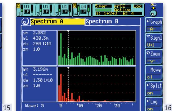
16 Frequency spectrum for current, voltage (as bar chart), with CE-limits, linear or logarithmic
