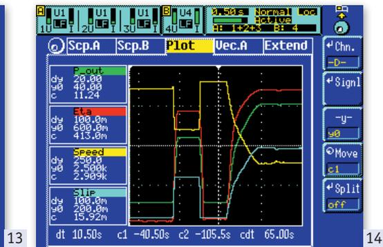
14 Plot display works like a strip chart recorder and can plot all measured or formula calculated values
