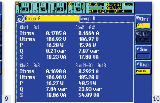
9 Large display with six important values of the frequency converter input, measured in group B
