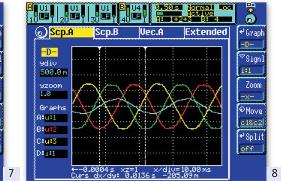
8 Scope display of the low pass filtered 3Ø output, the chopper frequency is no more contained because of being outside the filtered range
